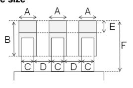
A=1.7+/-0.2mm B=2.6+/-0.2mm C=1.5mm (typ) D=2.0mm (typ) E=1.1mm (typ) F=4.8mmMax (typ: 4.3mm) E: Length of soldering area
